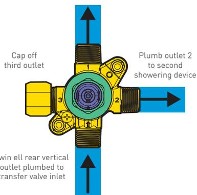
Twin ell rear vertical outlet plumbed to transfer valve inlet
