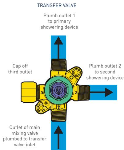
**IMPORTANT** - plumb showering outlets as valve diagram recommends. Plumbing 2 outlets will require capping port number 3.
