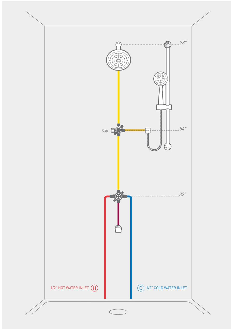
**IMPORTANT** - plumb showering outlets as valve diagram recommends. Plumbing 2 outlets will require capping port number 3.
